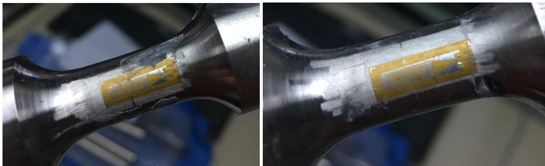
Fig. 56. Strain gauges still attached to the coupon after the second test.
