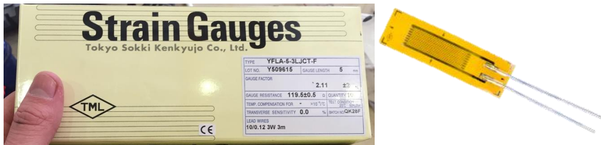
Fig. 36. Strain gauges box (left). Strain gauge (right).
