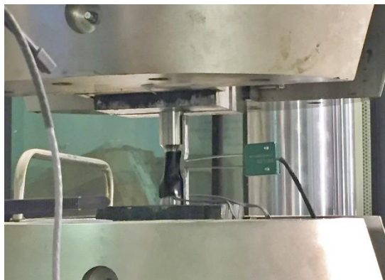
Fig. 44. Coupon with extensometer set up in the instron 8803.
