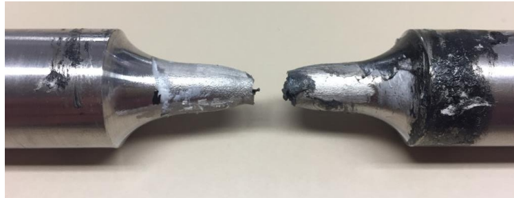
Fig. 55. Fractured Coupon from failed test.
