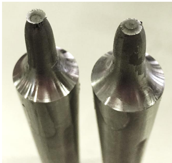
Fig. 53. Fractured coupon. Monotonic tensile test.
