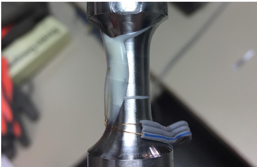
Fig. 57. Strain gauge attached with two component EA-2A adhesive.
