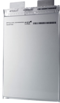
Figure 4.1: Picture of the lithium-ion pouch cell studied in this work.
