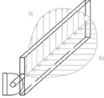
Figure A.16: Simplified scheme of the normal and tangential forces ( source: self elaboration ).
