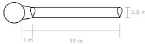
Figure 1.6: Scheme of the blade we have used in our model, according to the simplifications that have been set out in this chapter ( source: self elaboration ).
