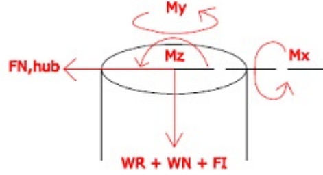
Figure 2.40: Summary of the efforts transmitted from the nacelle onto the tower ( source: self elaboration ).
