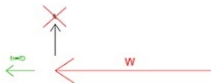
Figure A.25: Relative wind speed for a stopped windmill ( source: self elaboration ).
