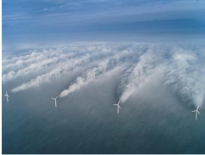
Figure 1.13: In this photograph we have tried to introduce the idea that the presence of other windmills may interfere on the activity of a particular windmill belonging to a wind farm ( source: http://nanosync.wordpress.com/ ).
